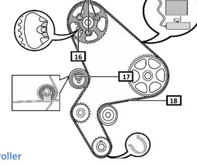
31) Unscrew and remove the idler roller
