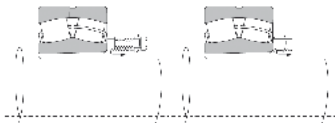
Removal of Withdrawal Sleeve with Withdrawal Nut
