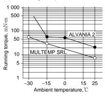
Starting torque and running torque are lower with MULTEMP SRL grease than with ALVANIA 2 grease.
