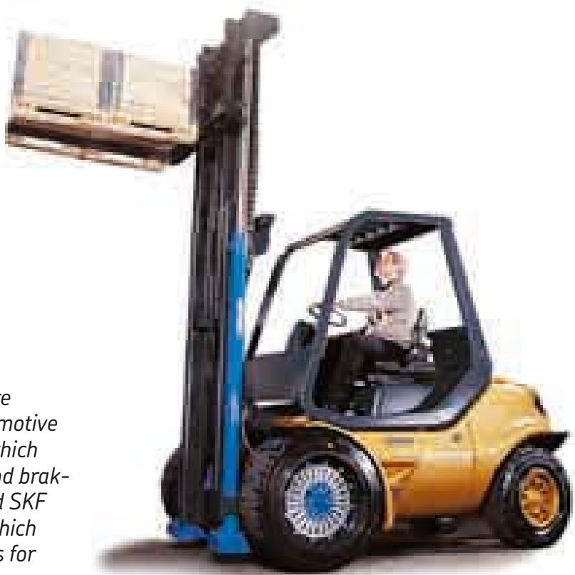
*SKF is also a leader in automotive by-wire technology, and has partnered with automotive engineers to develop two concept cars, which employ SKF mechatronics for steering and braking. Further by-wire development has led SKF to produce an all-electric forklift truck, which uses mechatronics rather than hydraulics for all controls.*
