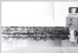
Before passage of ball slide (Significant foreign matter remains)
