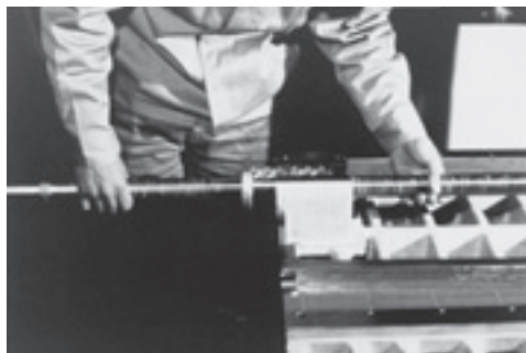
Photo 14.4 Installation of ball nut
