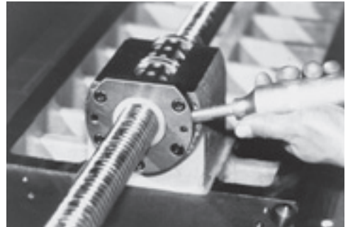
Photo 14.7 Replenish lubrication grease
