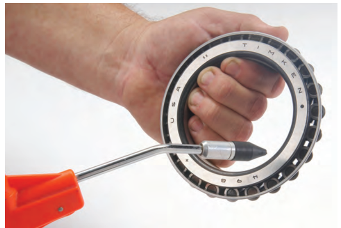
Fig. 19. Drying a bearing.
