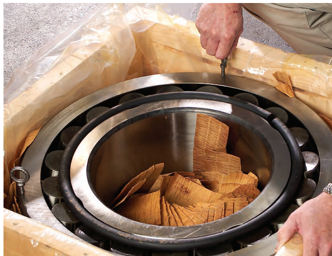
Fig. 2. Eyebolts can be inserted into lifting holes.
