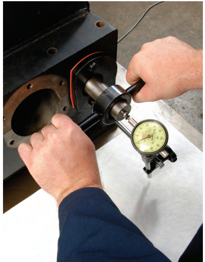
Fig. 27. Measure axial movement by locating a dial indicator against the end of the shaft.
