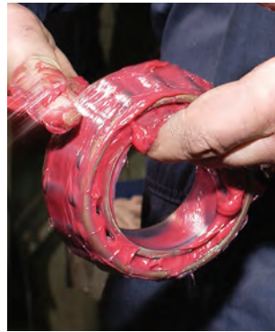
Fig. 58. Grease can easily be packed by hand.
