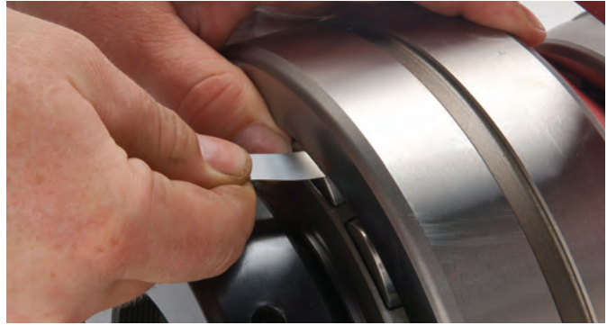
Fig. 30. Measure of RIC before installation.
